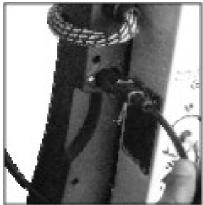
(10) Put the fan plug into the designated socket which is at the back side of the generator.
